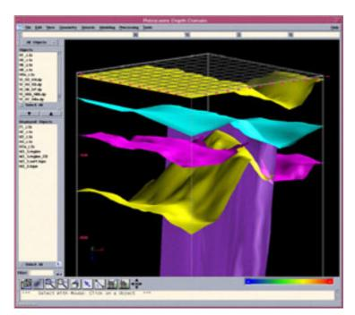
Also in GeoCaem it is possible to plan acquisition with further ray tracing in order to obtain the optimal spread of sources and receivers for field acquisition.
