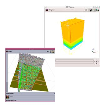
GeoINT 3D provides a three-dimensional view of different types of information: seismic sections (2D and 3D), horizons, wells - by simple dragging of the required object from any window to the 3D window. In GeoINT virtual reality visualization is possible. Using standard stereo glasses you can find yourself inside the created model.
